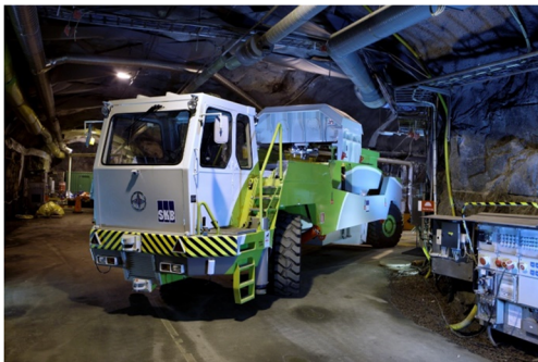
Fig. 11. (a) Tests in the Äspö Hard Rock Laboratory to demonstrate the deposition of a dummy canister and (b) the installation of bentonite backfill blocks. Source: courtesy of SKB.
