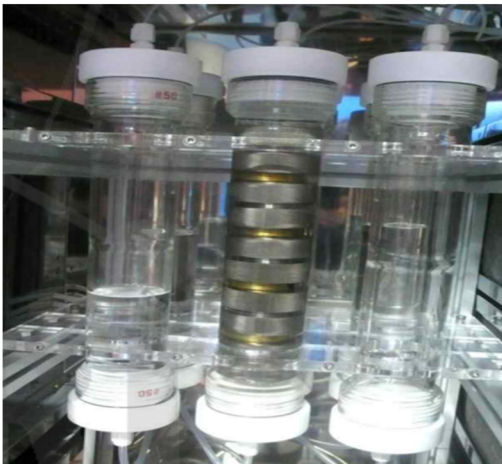
Fig. 9. (a) Test chambers in the KAERI Underground Research Tunnel facility measuring the corrosion of copper and (b) placement of instrumentation in a buffer of pre-compacted bentonite blocks as part of the engineered barrier system test in the Horonobe URL. Source: (a) courtesy of KAERI and (b) courtesy of JAEA.
