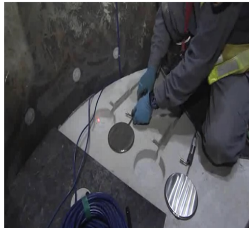
Fig. 9. (a) Test chambers in the KAERI Underground Research Tunnel facility measuring the corrosion of copper and (b) placement of instrumentation in a buffer of pre-compacted bentonite blocks as part of the engineered barrier system test in the Horonobe URL. Source: (a) courtesy of KAERI and (b) courtesy of JAEA.
