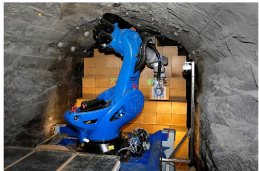
Fig. 11. (a) Tests in the Äspö Hard Rock Laboratory to demonstrate the deposition of a dummy canister and (b) the installation of bentonite backfill blocks. Source: courtesy of SKB.
